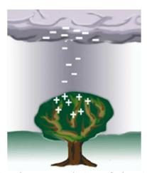
Fig. 3: The accumulation of electric charges must be great enough to overcome the insulating properties of the air. When this happens, a stream of negative charges pours down toward a high point where positive charges have clustered due to the pull of the thunderhead.
